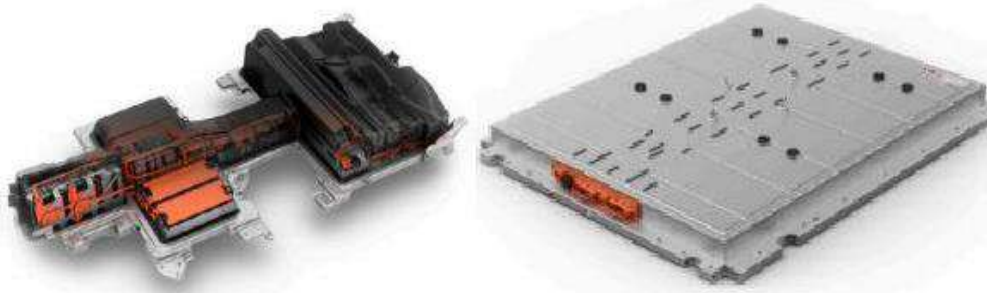
Fig-2. 4 Comparison of VW MQB and MEB battery packs used as reference for modular design.
